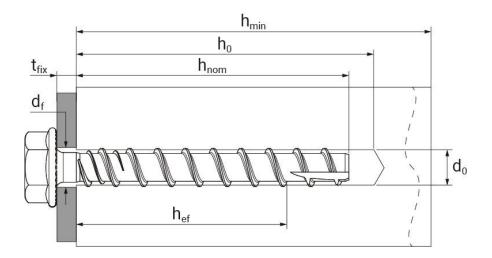
$h_{min}$  : Minimum thickness of member  $d_0$  : Nominal drill hole diameter
